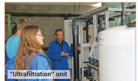
Membrane manufacturers participated in this pilot unit with 2 modules that are already operating (Aquasource and Polymem) and two others that will be installed later (X-flow and Hydranautics).
